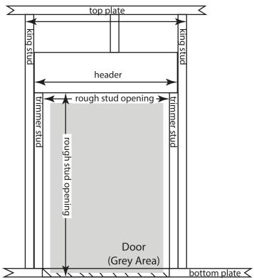
Please note that the bottom plate of a door is cut out between the trimmer studs before the door is hung.
